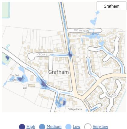
Figure 52: Extent of surface water flooding
