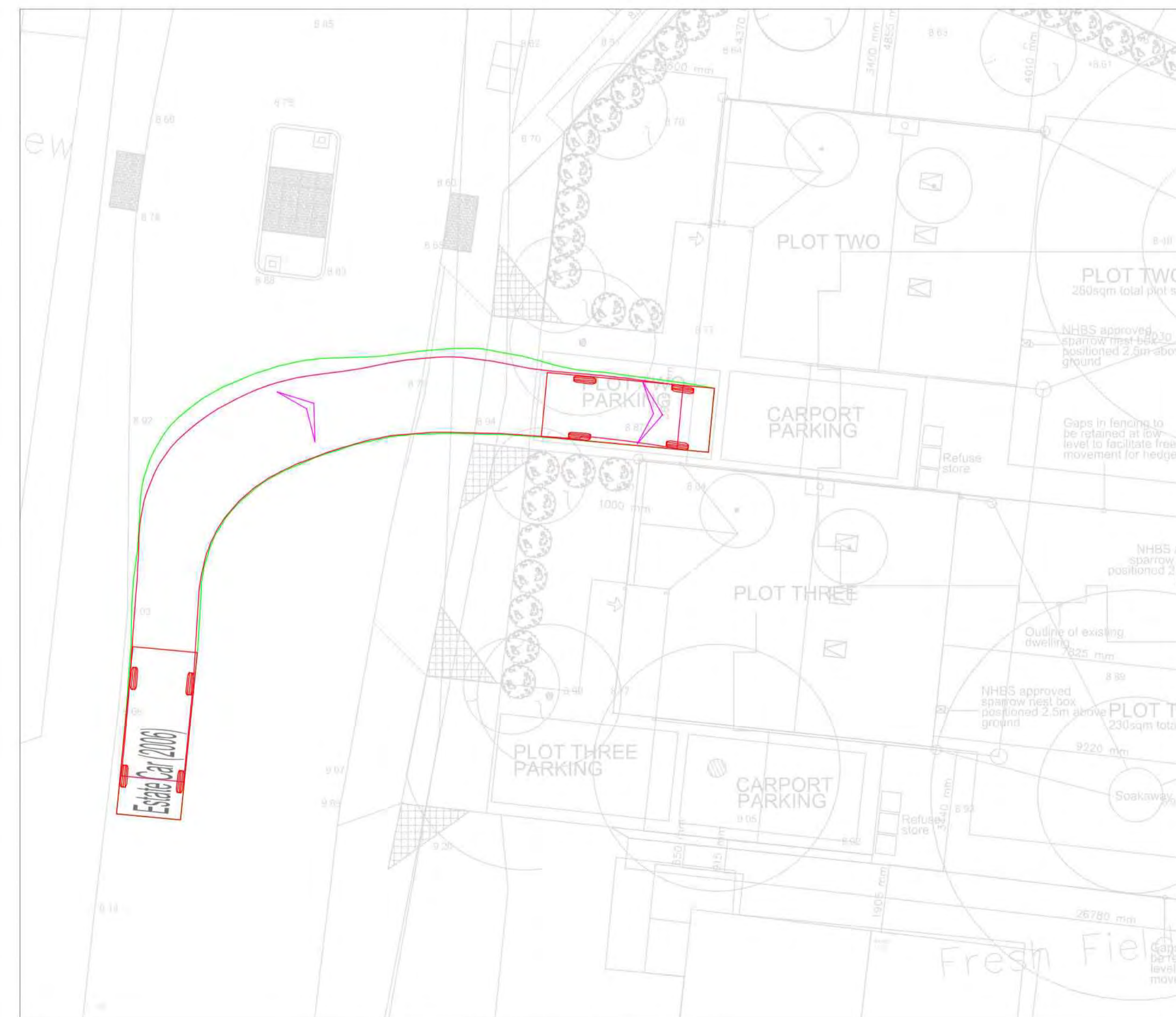
Swept Path - In - Forwards Direction Far side
