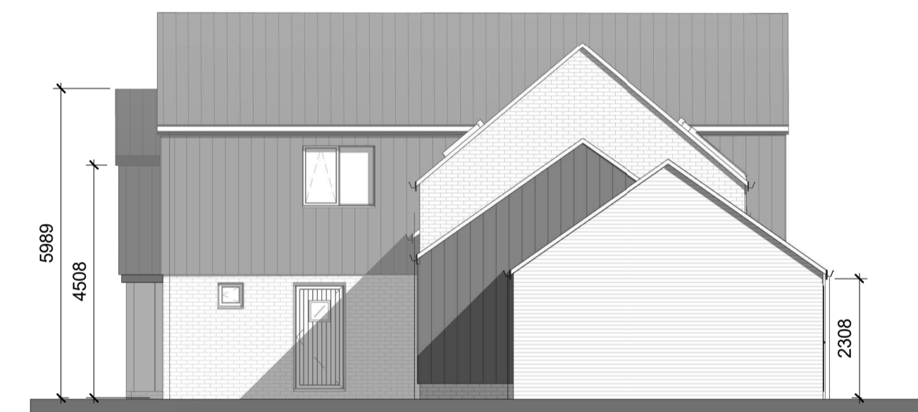
1:100 North Elevation (Side)
